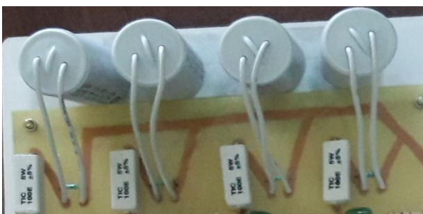
Capacitor bank and the resistors used in project
