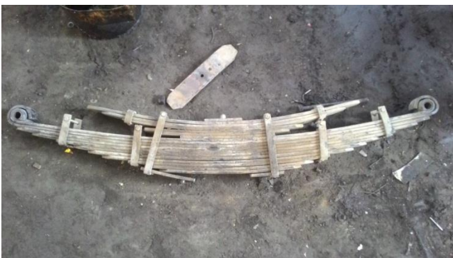
Fig. 7-failure due to bending effect on leaf spring
