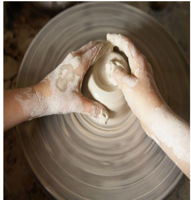
Fig. 2- Centering process in throwing [3]
