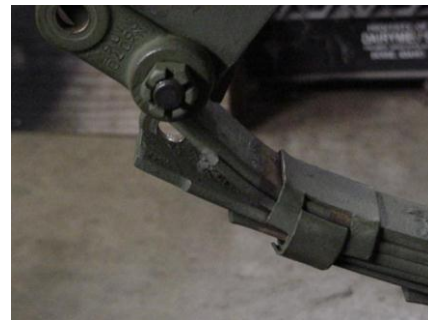
Fig.1- Bending effect on leaf spring
