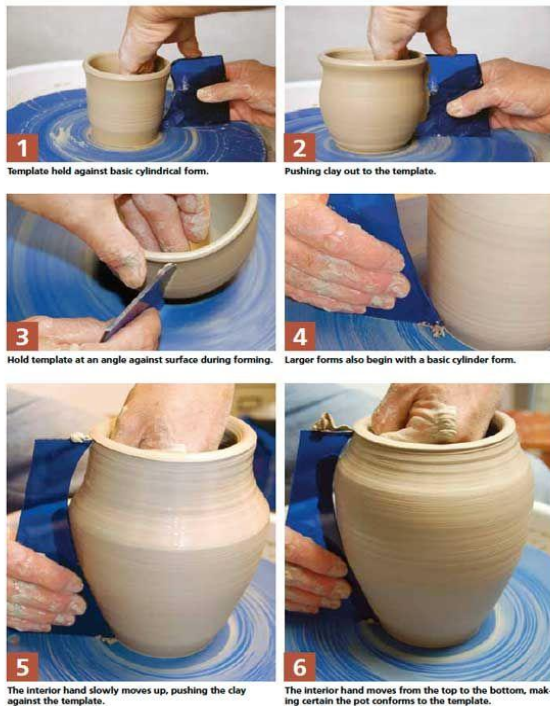
Fig. 1- Throwing on potter's wheel [2]
