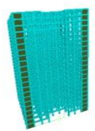
Fig. 1 Rendered view of STAAD.Pro model with shear wall
